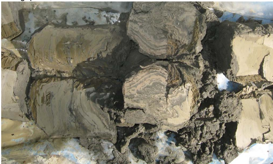
Folded varves observed in several core samples corresponded with failure surface elevations observed in existing inclinometers.
