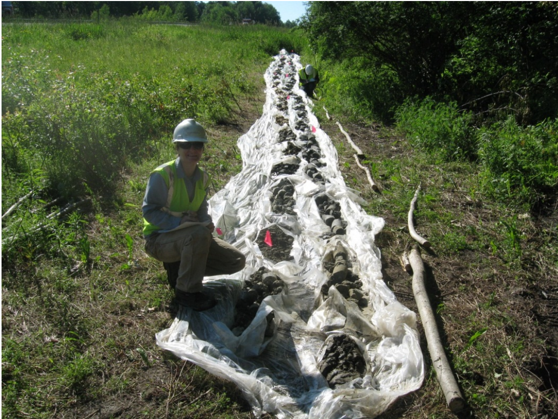
Sample logging activities of sample cores obtained from a single borehole.
